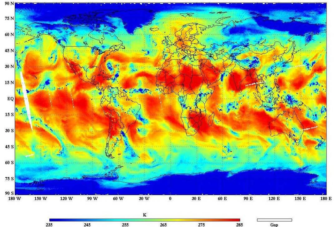
First global image of ATMS channel 18 microwave antenna temperature at 183.3 GHz acquired on November 8, 2011
