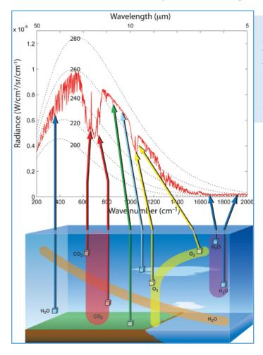
Figure 3 The thermal IR spectrum. Frequency is in wavenumbers (cm<sup>-1</sup>), radiance in W cm<sup>-2</sup> sr<sup>-1</sup> (cm<sup>-1</sup>)<sup>-1</sup>. Water vapor exhibits strong, narrow lines in the frequencies intervals 200–550 and 1100–1500 cm<sup>-1</sup>. Carbon dioxide absorbs in its  $\nu_2$  band in the frequency interval 550–770 cm<sup>-1</sup>. The area under this curve measures the flux of thermal IR energy radiated to space, thus cooling the Earth system.
