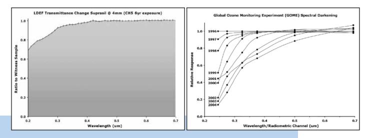
Figure 19 Changes over time: (a) Long Duration Exposure Facility transmission of optics caused by in-orbit contamination layers and (b) GOME.
