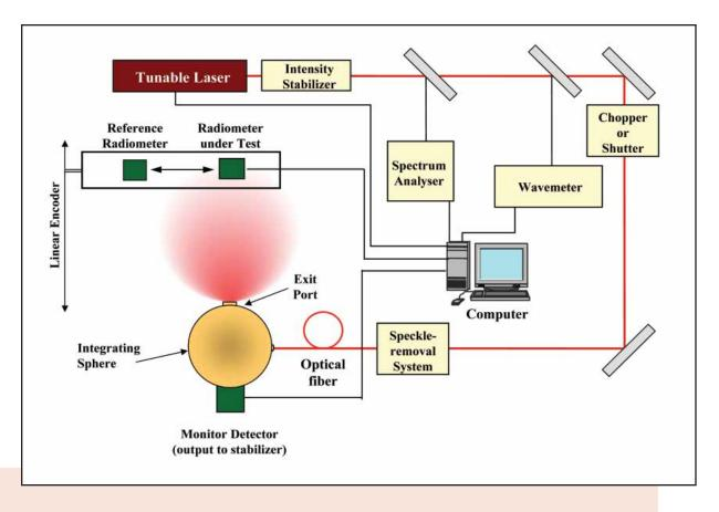
Figure 9 Schematic diagram of the NIST Spectral Irradiance and Radiance Responsivity Calibration using Uniform Sources (SIRCUS) Facility.
