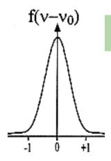
Figure 35 The lineshape for a single channel of a generic spectrometer.
