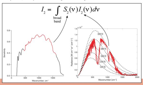
**Figure 33** Aging due to environmental exposure causes alteration of the radiometer spectral response function. Since the unknown climate change signal is convolved with this unquantified change in spectral response function, definitive detection and interpretation of climate change is out of reach.
