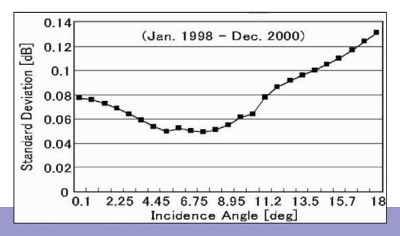
Figure 23 Standard deviation of monthly radar cross sections of rain-free sea surface at different incidence angles derived from the TRMM/PR measurements. The data include 36 months of data taken from January 1998 to December 2000. The standard deviations include both the natural variations of sea surface cross sections and the variations of radar sensitivity. The data show that the long-term stability of the radar itself is better than 0.05 dB. (Okamoto et al, 2002)
